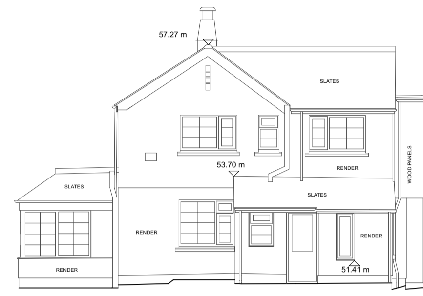
5 South west Elevation 1:100
