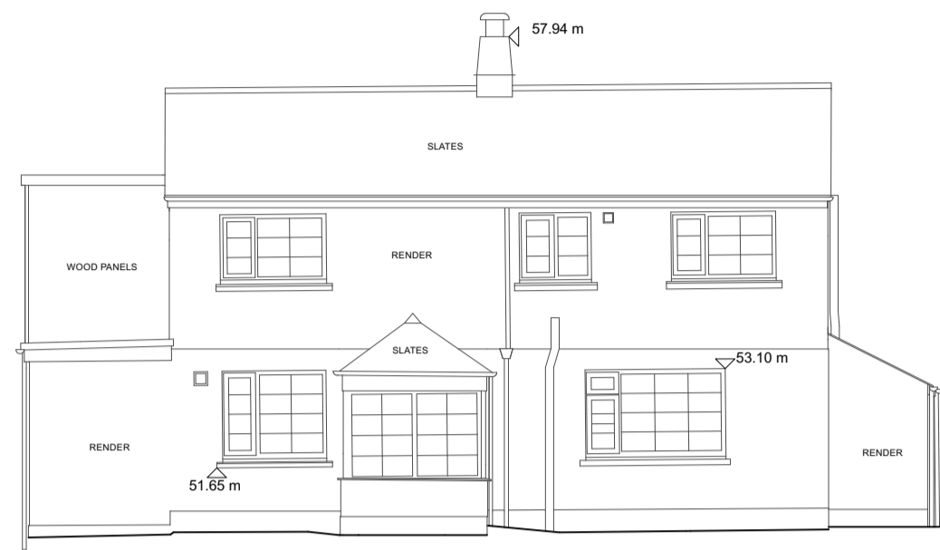
2 North west Elevation 1:100
